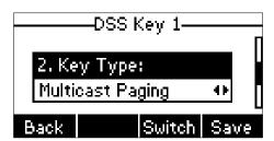
5. Enter the multicast IP address and port number (e.g., 224.5.6.20:10008) in the **Value** field.
