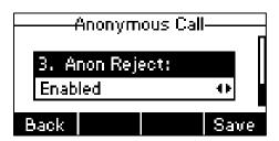
5. (Optional.) Enter the anonymous call rejection on code and off code respectively in the **On Code** and **Off Code** field.
